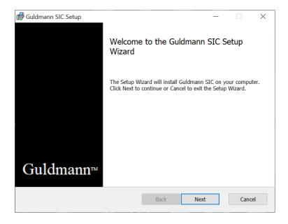
If you are a certified Guldmann technician, check the "**Technician version**" installation option to obtain access to the advanced program options. Type your full name before proceeding. This option requires a special activation code. Contact Guldmann to obtain the activation code.
