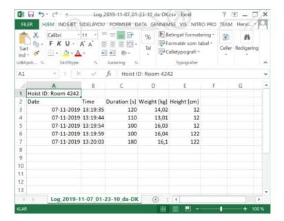
**Note:** The weight measures stored in CLM are generated during a lifting cycle, and they do not represent an actual controlled weighing. Therefore, any weight shown in the CLM can only be used as an indication regardless the hoist is equipped with weighing module or Class III scale module.
