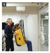
When the Combi-lock has engaged position yourself behind the user and push lengthwise the traverse rail though the Combi-lock. The user is still facing / looking lengthwise the traverse rail.
