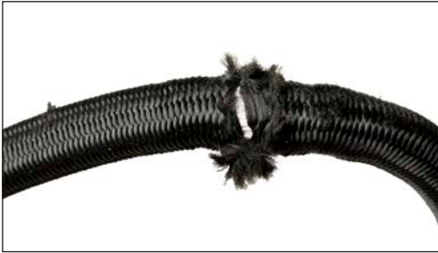
Example of a defective line
